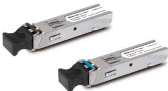
The MGB family consists of Small Form Factor Pluggable (SFP) transceiver modules that are specifically designed for high performance integrated duplex data link over single mode optical fiber. These transceiver modules are compliant with the SFP Multisource Agreement (MSA) and hot pluggable. These modules offer an easy way to be installed in SFP MSA compliant ports at any time without the interruption of the host equipments operation.
